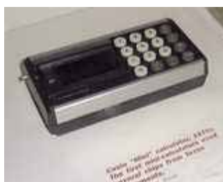
early transistor calculators - Casio "Mini" used chips from TI (left); TI SR-10 calculator showing circuit in transparent case, used a single chip 1972, from Smithsonian NMAH
