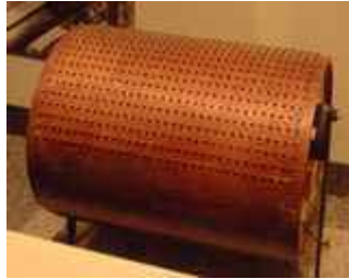
magnetic drum memory of the Atanasoff-Berry Computer 1939, from Smithsonian NMAH
