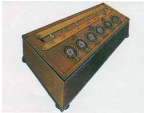
Figure 1.3 – Adding Machine, In 1642, Blaise Pascal
